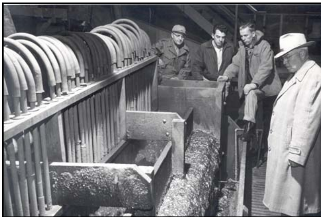
Froth flotation forms a bubbly mix of valuable ore minerals.
